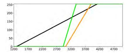
14-bit to 8-bit (linear) mapping function of min/max normalization. Grid-wise normalization shows narrower range and steeper slope.
